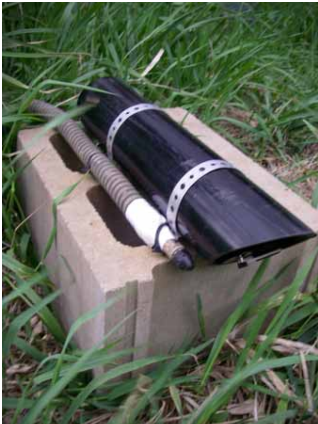
DTS-12 paired with a Druck pressure transducer (stage monitoring device) – ready to be deployed.
