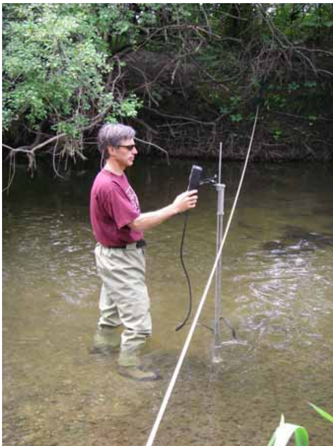
DTS-12 paired with a Druck pressure transducer (stage monitoring device) – ready to be deployed.
