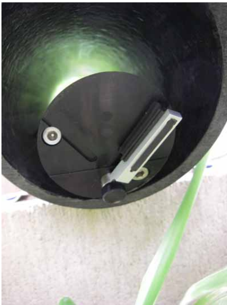
Looking into the eyes of a DTS-12 (turbidity sensor). The rugged wiper cleans the lenses regularly to prevent fouling by periphyton.
